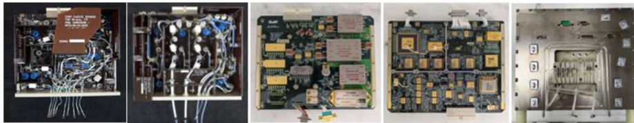
Fig. 13 From left, CoDICE HVPS 1, HVPS 2, LVPS, CDH, and the Ebox
